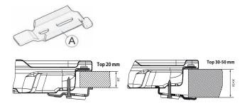
Where the hob is not installed over a built-in oven, a wooden panel must be installed as insulation. This must be placed at a minimum distance of 20 mm from the lower part of the hob.
