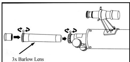
Your telescope also comes with a 3x Barlow Lens which triples the magnifying power of each eyepiece. However, the greatly magnified images should only be used under ideal conditions – see the Calculating Magnification section of this manual. To use the Barlow lens remove the diagonal and insert the Barlow directly into the focuser tube. You then insert an eyepiece into the Barlow lens for viewing.
