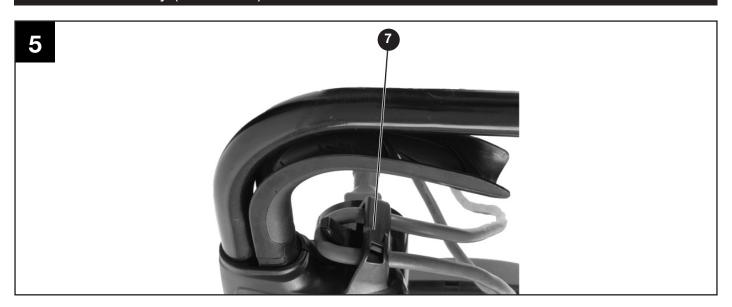
Hook the cable through the cable strain relief hook 7 to help prevent it from coming loose or disconnected whilst you are mowing. (Fig. 5)
