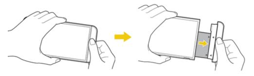
3. Hold the battery and module with both hands and separate them from one another in an outward arc (as indicated below) to disconnect the battery terminals.
