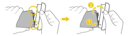
3. Push the battery module all the way into the device.
