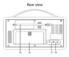
15. Telescopic antenna 16. Battery compartment
