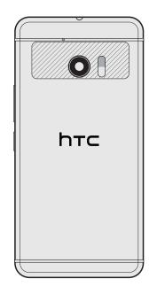
Make sure that the NFC area (shaded part) of HTC 10 and the other phone's NFC area are close to one another. Experiment by slightly moving the phones until a connection is made.
