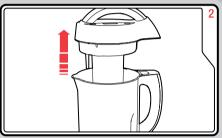
Remove the Lid (2), be careful not to touch the Serrator Blade (8). WARNING: Sharp Blades
