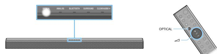
Press the OPTICAL button to turn on the OPTICAL indicator. Then, press the  $\checkmark$  (volume) button to adjust the volume. If you connected your TV to the ANALOG jack in step 1, press the ANALOG button.
