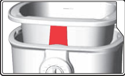
The Thermostat Pad (shown above) is located on the side of the Pan. Greasy deposits in this area cause the Intellechef Multicooker to misread the temperature of the Pan and overheat. When cleaning the Pan ensure the pad is cleaned thoroughly and free of any grease or food deposits.
