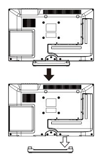
Use the four screws provided to fix the TV onto a wall mounting bracket (not included) via the four VESA standard holes on the back of the television. Wall-Mounting Screws
