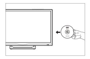
If play does not start automatically, press the "  $\blacktriangleright II$  " button on the remote control, or the "  $\triangleright II$  " button at the righ t of the TV.
