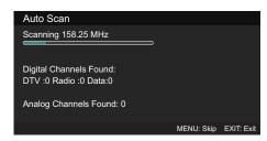
6. If you want to skip the DTV tuning, press the **MENU** button to interrupt the tuning half way. You will then go straight to ATV tuning. You may repeat the above step if you also want to skip the ATV tuning.
