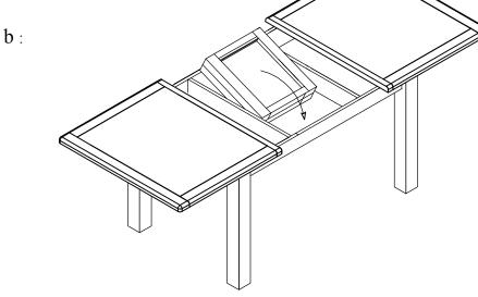
c: Hold the top of table to push on both sides of table as shown by the arrows. Use safety locks to ensure table top will not move while using ( see safety lock instruction below)
