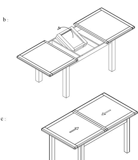
c :Hold the top of table to push on both sides of table as shown by the arrows. Use safety locks to ensure table top will not move while using ( see safety lock instruction below )
