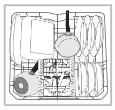
Very soiled dishes and pans should be placed in the lower rack because in this sector the water sprays are stronger and allow a higher washing performance. Several dishwasher models are fitted with tip-up sectors<sup>\*</sup>. They can be used in a vertical position when arranging dishes or in a horizontal position (lower) to load pans and salad bowls easily.
