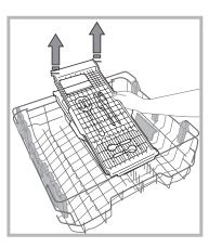
The upper rack can be adjusted for height based on requirements: high position to place bulky crockery in the lower rack and low position to make the most of the tip-up compartments/sectors by creating more space upwards.
