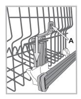
If the rack is equipped with a **Lift-Up device**<sup>\*</sup> (see figure), lift it up by holding its sides. To restore the lower position, press the levers (**A**) at the sides of the rack and follow the rack down.
