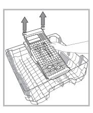
The upper rack can be adjusted for height based on requirements: high position to place bulky crockery in the lower rack and low position to make the most of the tip-up dispensers/sectors by creating more space upwards.
