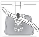
The lower spray arm can be removed by pressing on the side tabs and pulling it upwards.
