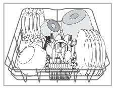
Very soiled dishes and pans should be placed in the lower rack because in this sector the water sprays are stronger and allow a higher washing performance.
