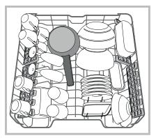
Several dishwasher models are fitted with tip-up sectors<sup>\*</sup>. They can be used in a vertical position when arranging tea/ dessert saucers or in a lower position to load bowls and food containers.
