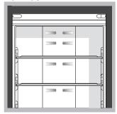
The No Frost system circulates cold air continuously to collect humidity and prevent ice and frost formation. The system maintains an optimal humidity level in the compartment, preserving the original quality of the food, preventing the food from sticking together and making defrosting a thing of the past. Do not block the aeration cells by placing food or containers near the refrigerating back panel.
