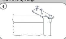
Before reassemble the hinge to the left side, reverse the direction of the hinge.
