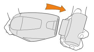
To remove the Motorised Tool (18v Gator only) for cleaning or when not in use, gently twist down and pull to detach.
