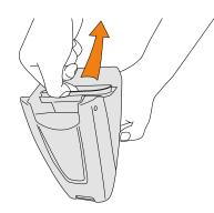
Whilst holding the dirt container over a bin, grasp the filter gently and pull out.
