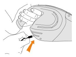
Plug charger into the mains and insert lead into back of machine. Initial charging time is 24 hours.
