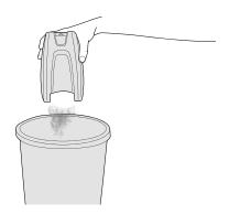
Shake any excess dirt or debris from the dirt container.
