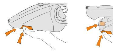
To empty the dirt container, press both buttons either side of the dirt container to release lid.
