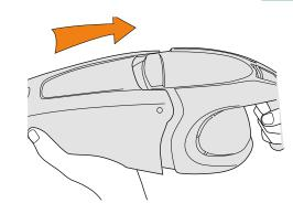
To re-attach the dirt container, align bottom of the dirt container and push until it locks into place.
