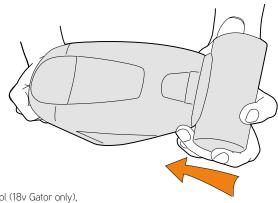
To attach the Motorised Tool (18v Gator only), align with dirt container and push until it locks in place.
