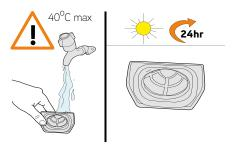
Wash the filter under running water and leave to fully dry for a least 24 hours before replacing.
