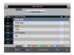
To rename a channel, press the "UP/DOWN" button to choose the channel to be renamed. Press the BLUE button to enter the channel rename page. This is shown below:
