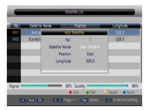
Use UP/DOWN arrows to select the different properties in the add satellite dialogue box. To change a property eg, such as "Satellite Name" Highlight and press ">" right arrow button which brings up a rename box. Use UP/DOWN, LEFT/RIGHT arrows to select characters.
