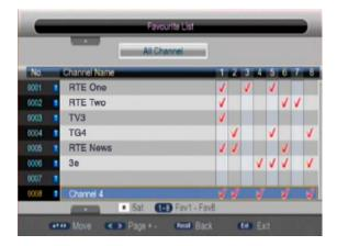
Press UP/DOWN, LEFT/RIGHT button to choose the channel to be selected, then press the numbered keys 1-8 on the remote control to set different favourite lists. Terrestrial and Satellie channels can be stored in the same Favourites list.
