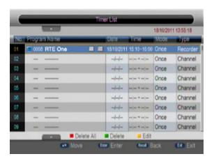
The Timers menu provides a list where timers can be added, viewed, edited or deleted. The list displays both manually added and scheduled timers set via the EPG. A maximum of 99 timers can be set.
