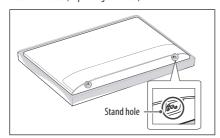
When attaching a wall mounting bracket to the TV, insert the wall mount spacers into the TV wall mount holes to adjust the vertical angle of the TV. (Only when the item of the following form is provided)
