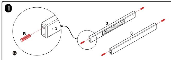
• Insert Wooden Pins (B) into the top hole on the Side Rails (3) on both ends. Repeat for other side rail.
