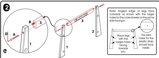
• To attach the **Side Rail (3)** to the **Legs (1 & 2)** simply line up the wooden pins you inserted in Step 1 into the top hole on the flat surface of the legs. Ensure that you have one (1) leg and one (2) leg as shown in image. Bolt together using the **55mm Allen Head bolt (A)** tightening with **Allen key (D)**. Repeat for other side.
