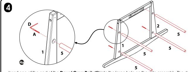
Insert one of the end of the Dowel Cross Rails (5) into the large hole on the side assembly. The dowel should go into the hole tightly as shown in 4a. Some gentle tapping may be required. Bolt the dowel into place with a 55mm Allen Head Bolt (A) and tighten in place. Repeat for the three other ends of the dowels.
