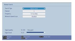
After selecting search type as **Digital Aerial**, you can enter the multiplex or frequency number using the numeric buttons and press **OK** button to search.
