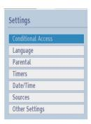
Press **Up** or **Down** button to highlight a menu item. Press **OK** button to select an item. Press **MENU** button to exit.
