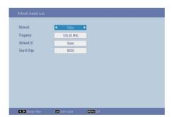
You can select **Network**, **Frequency**, **Network ID** and **Search Step** from this screen. For highlighting lines you see, use **Up** or **Down** button. You can set **Search Step** as 8000 kHz or 1000 kHz. If you select 1000 kHz, the TV will perform search process in a detailed way. Searching duration will thus increase accordingly. When finished, press **OK** button to start automatic search.
