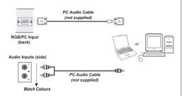
To use a PC, set the monitor output resolution on the PC before connecting it to the TV. To display the optimum picture, use the PC setting feature.
