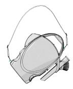
To carry in a horizontal position: clip one end of the shoulder strap into carry handle slot. Clip the opposite end into the bottom of the vacuum slot.
