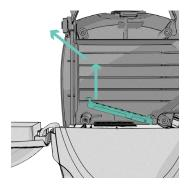
Lift up on the finger tab and pull out.
