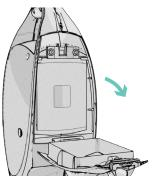
Rotate the inner bag door down.
