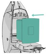
Insert a new inner bag by fitting the cardboard rim between the tabs inside the bag holder.
