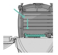
Insert the frame back in. Then insert the inner bag back into place, and close the door.
