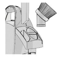
Load the tools onto the tool caddy.
