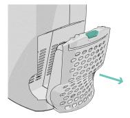
Push down the HEPA filter door tab to pull out
