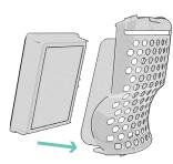
Slide the HEPA filter up and out. Insert a new filter by aligning the slots on the side of the filter with the tabs on the filter door. Place the HEPA filter door back in until it snaps into place.
