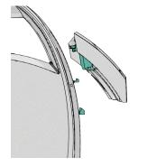
Align the middle slot and two pronged tabs with the vacuum tab and slots.
