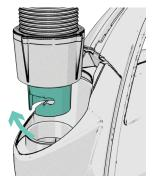
Align the J-shaped slot at the end of the hose with the tab inside the hose inlet. Turn clockwise to lock into place. Attach the tool you would like to use. Twist and push to lock in. Twist and pull to remove.
