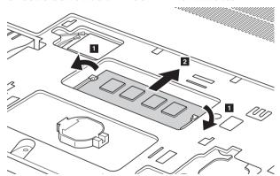
(a) Align the notch of the DDR3 SDRAM with the protrusion of the socket and gently insert the DDR3 SDRAM into the socket at a 30-45° angle.
