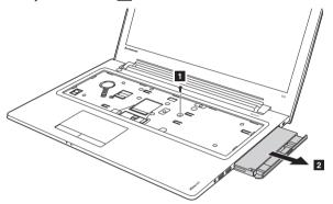
4 Remove the screw 3, then remove the optical drive bracket in the direction shown by arrow 4.
