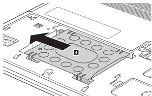
6 Take out the hard disk drive secured in a metal frame 5.
