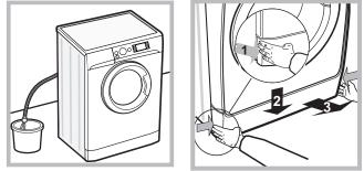
2. make sure the water level inside the machine is lower than the door opening; if it is not, remove excess water using the drain hose, collecting it in a bucket as indicated in the figure. 3. remove the cover panel on the lower front part of the washer-dryer (see figure).
