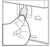
4. pull outwards using the tab as indicated in the figure, until the plastic tie-rod is freed from its stop position; pull downwards and open the door at the same time. 5. reposition the panel, making sure the hooks are securely in place before you push it onto the appliance.
