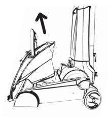
4. Rinse the tank and filter with warm water (max 40°C). Wipe and let dry fully before storing to prevent mildew. Replace the dirty water tank lid.
