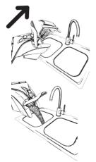
2. Hold the handle and pull tank up and out.
