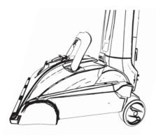
2. Tilt carpet washer backwards and line up tabs under nozzle with front of base on carpet washer.
