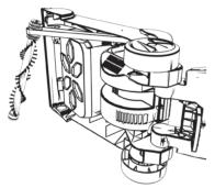
3. Line up brushbar with base, push into place. Make sure the brushbar ends are in the correct orientation (A). 2. Place the new belt onto the spindle, place other end of belt on rounded area of brushbar without bristles.
