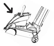
4. Now place the rear of the tank into the base of the cleaner. Push handle down until it clicks.
