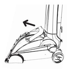
3. Lift to remove the dirty water tank lid. Empty the dirty water over the sink and rinse under water.
