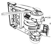
4. Replace belt cover and secure with the three screws.
