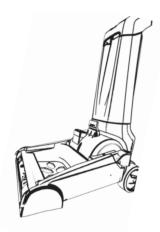
3. The nozzle should be flush with the base. If it's not, this will result in poor water pickup.
