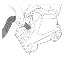
2. Line up tabs on hose into hose connection port. Push and twist hose clockwise to lock into place.
