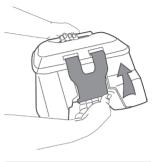
3. Lift dirty water tank clip up and outward to release.
