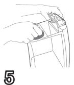
Twist clean water tank cap anti clockwise to remove.
