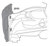
3. Line up tabs on nozzle with holes in carpet washer. Slide tabs into holes, press down on nozzle until clicks into place.
