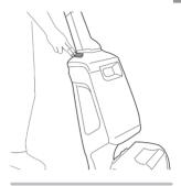
3. Press the on/off button to switch on. Select WASH on mode selector switch (No water/solution will be delivered on RINSE mode).
