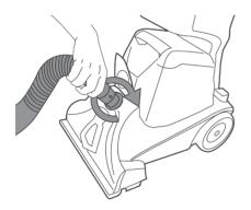
3. Line up solution tube connector with solution tube connection port. Push and twist clockwise to lock into place.
