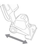
5. Squeeze trigger on the forward stroke, release trigger on backward stroke to recover solution/water.
