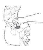
4. Empty dirty water over the sink. Rinse dirty located at the back of water tank and lid under water to remove debris.
