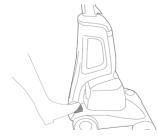
4. Press the Max Extract pedal to de-activate the Max Extract mode.
