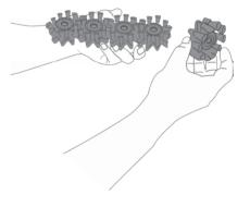
1. Pull firmly to unclip each side of Power Scrub cover (one side at a time). 2. Remove individual brushes, clean and rinse under running water to remove debris.
