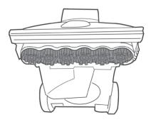
3. Remove any threads or hair caught around the brush, rinse under water to remove debris.
