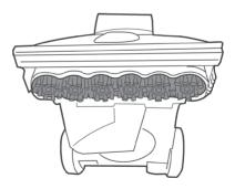
3. Refit the individual brushes. Line up tabs on Power Scrub cover with tabs on brush frame. Push and clip covers until click into place. 4. Leave to fully dry. Line up tabs on side of Power Scrub cover with carpet washer, push firmly until clicks into place.
