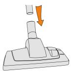
Insert the other end of the telescopic tube into the floorhead.
