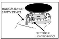
you must hold the control knob in for about 3-7 seconds after the burner has been lighted to allow the gas to pass until the safety thermocouple has heated.
