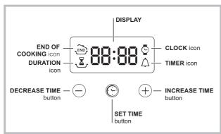
! The Top Oven and Main Oven can be controlled by the automatic timer. When the timer control has been set for one oven, it is possible to use the other oven only during the same automatic cooking programme.
