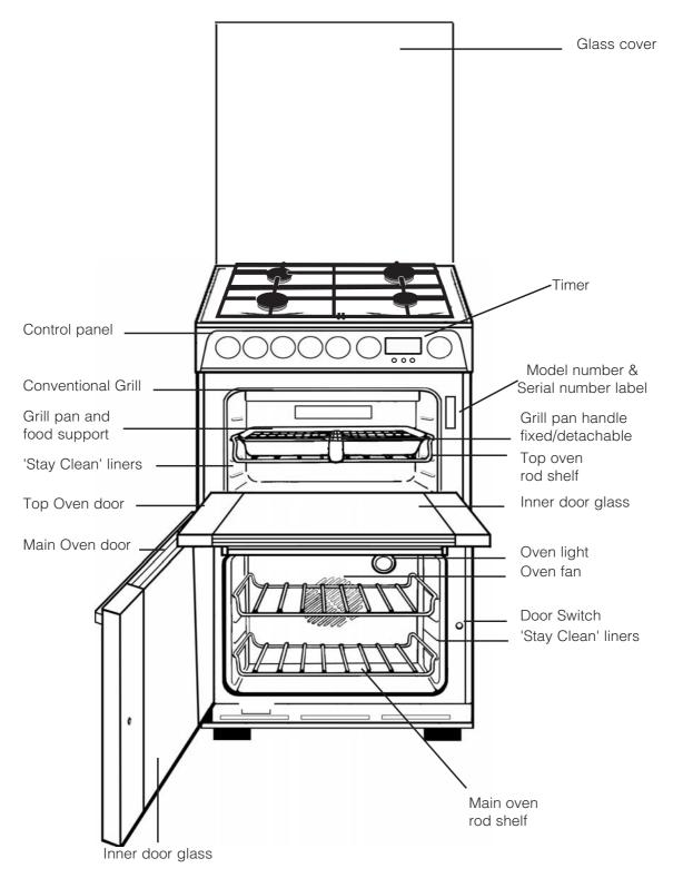
NOTE: To keep the controls cool when the appliance is used, a flow of air may be blown from beneath the control panel. If the appliance is still warm, this cooling fan will run on when all controls have been turned off. This is normal and is not a fault.
