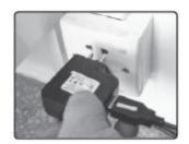
**NOTE**: While charging the battery, the LED light turns on. The battery is fully charged when the LED light turns off.
