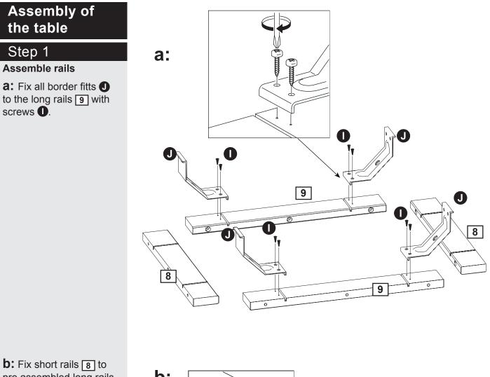
pre assembled long rails with screws **①**.
