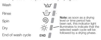
**Note:** during the "Drain" phase, the indicator light corresponding to the "Spin" cycle phase will illuminate.
