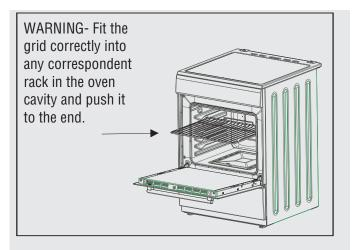
To locate grid correctly in the cavity, put it to any rack and push the grid up to the end.
