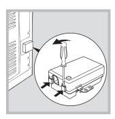
1 Open the terminal board by inserting a screwdriver into the side tabs of the cover. Use the
