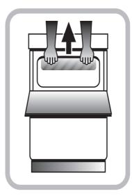
The height of the cooker can be adjusted by means of adjustable feet in the plinth (900mm - 915mm). Adjust the feet by tilting the cooker from the side. Then install the product into position. NOTE: This appliance must not be fitted on a platform.
