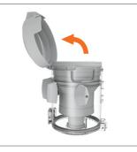
Push the tab on the lid of the dirt container and lift the cover to access the filter.
