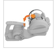
To refit, line up the dirt container connection with the handheld handle. Push the dirt container back onto the handle until it clicks into place.
