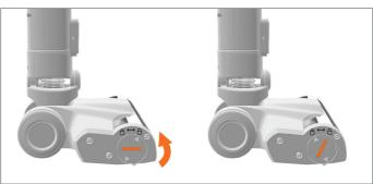
Using a coin, push and turn the brushbar lock anticlockwise to release the brushbar.
