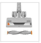
Clear any dirt/debris from the end caps and inside the housing of the powered floorhead.
