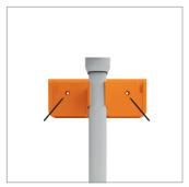
Holding the wall bracket securely against the wall, make a small mark for each screw. Secure the wall bracket to the wall using the wall plugs and screws.
