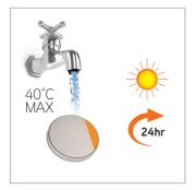
Wash the filter under running water (40°C max). Leave for at least 24hrs or until fully dry before replacing.
