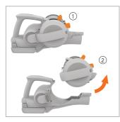
Squeeze the latch on the dirt container to release.
