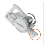
Press the handheld release button and remove the reach wand. Check and clear any dirt and debris from the handheld connection point.
