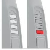
When the machine is in use the battery level indicator lights will illuminate indicating how much charge is remaining. When less than 20% charge is remaining the bottom light will flash red indicating the battery is running low and charging is required.
