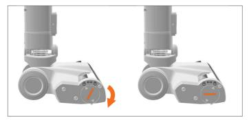
Refit the brushbar into the floorhead. Align the arrow on the brushbar cover so it points north, firmly push and twist clockwise to lock.
