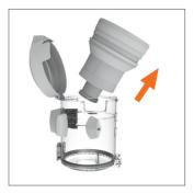
Lift the filter and separator from the dirt container.
