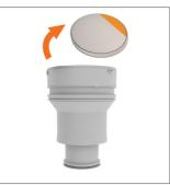
Pull the tab on the filter to remove from the separator.
