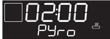
2. The duration of the Pyrolytic cycle will appear on the display.
