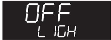
To stop the appliance from automatically deactivating the light after one minute, set this mode to **OFF**.
