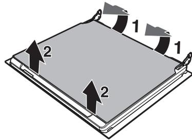
3. Some models are fitted with a pair of intermediate glass panes. Remove the intermediate glass panes by lifting them upwards.
