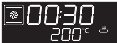
Each time the programming knob is pressed during a function, the parameters will be cycled through in the following order.
