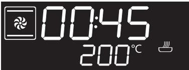
3. Press the programming knob a fourth time. The
