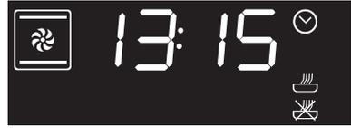
5. At the end of the cooking, STOP flashes on the display and a buzzer will sound that can be deactivated by opening the door or pressing/turning one of the two knobs.
