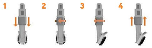
Push and twist the rotation collar to select the most suited cleaning angle for the chosen tool. There are four positions on the rotation collar for easier cleaning.
