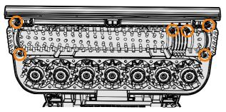
Refit belt guard and tighten x2 screws. Refit and tighten screws x2 on either side of side brushes. Refit SpinScrub brushes. Refit rug guard pins and tighten screws.
