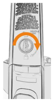
Turn handle lock dial clockwise to lock in position.
