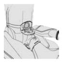
Push hose end and hose solution connector into hose and solution connection port.
