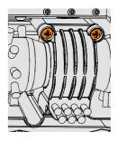
Use a crosshead screwdriver. Undo 2 screws and remove belt guard.
