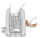
To recoil the remainder of the hose, secure the machine by holding the handle and turn the reel handle slowly.
