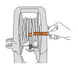
Once coiled, wrap the second velcro strap around the already coiled hose and secure.
