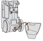
Unhook the solution tube and insert into the solution bag. Solution only dispensed with the trigger handle, lance and solution nozzle, or car/outdoor/rotary brush if supplied.
