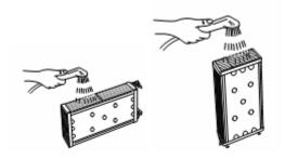
Whilst the condenser is removed, clean as much fluff as possible from inside the ducting by reaching a hand into the machine. In particular, keep the passage from the fan clear (on the right hand side of the condenser duct).
