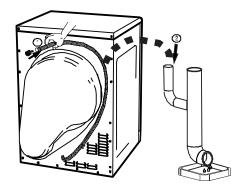
To return your drier back to taking the condensed water to the water bottle, simply fit the drain hose back to the valve at the top of your drier.
