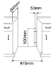
The illustration shows the minimum space required by the dryer and the position of the waste-pipe within this space and behind the dryer. If a trap is fitted it must not obstruct the air inlet at the back of the dryer. The waste pipe can be positioned on either side of the dryer.
