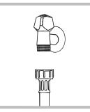
Connect the supply pipe by screwing it to a cold water tab using a 3/4 gas threaded connection (see figure).
