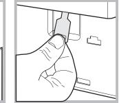
4. pull outwards using the tab as indicated in the figure, until the plastic tie-rod is freed from its stop position; pull downwards and open the door at the same time.
