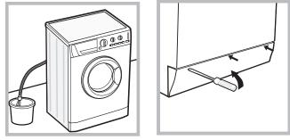
3. using a screwdriver, remove the cover panel on the lower front part of the washing machine (see figure).
