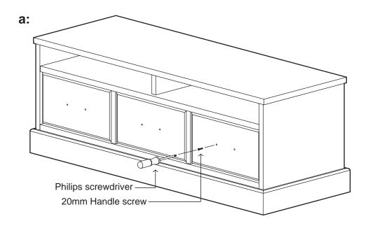
**b:** Replace the D handles on the front of the unit. Fix in position by screwing the 20mm handle screw into each handle from inside the unit using a Philips screwdriver.
