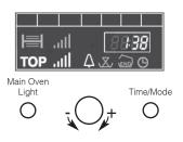
The minute minder can be cancelled at any time by following STEPS 1 and 2, setting the time period to zero using the +/- control knob.
