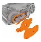
Pull to remove the belt cover Lift and separate brushbar and brushbar location plate. side cover. Remove belt.
