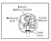
The wire coloured green and yellow must be connected to the terminal marked with the letter "E" or by the earth symbol + or coloured green and yellow. The wire coloured blue must be connected to the terminal "N". The wire coloured brown must be connected to the terminal marked "L".
