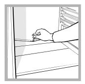
The refrigerator has an automatic defrosting function: water is ducted to the back of the appliance by a special discharge outlet (see diagram) where the heat produced by the compressor causes it to evaporate. It is necessary
