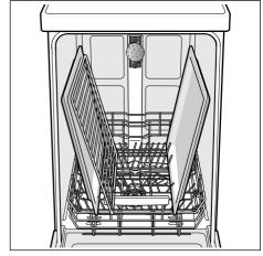
Large sheets or grilles and plates which have a diameter greater than 30 cm (gourmet plates, pasta plates, dinner plates) can be cleaned with the aid of the spray head. To do this, remove the top basket and insert the spray head as illustrated in the diagram.
