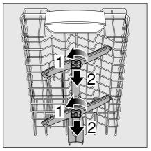
**3.** Remove the lower spray arm 24 upwards.
