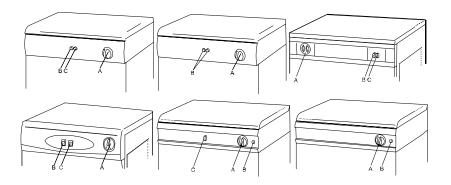
A. THE TIMER Select the required drying time based on the recommendations on the control panel.
