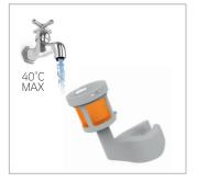
Wash the separator mesh under running water (40° max) to remove any dirt and debris
