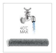
Rinse the brushroll in water (40  $^{\circ}$  max) and allow to dry before refitting.
