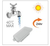
Wash the filter under running water (40°C max). Leave for at least 24hrs or until fully dry before refitting.
