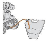
Unhook the solution tube and insert into the solution bag. Solution only dispensed with the trigger handle, lance and solution nozzle, or car/outdoor /rotary brush if supplied.
