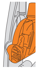
Line up TurboTool brushes into TurboTool holder, push into place until it clicks (some models only).
