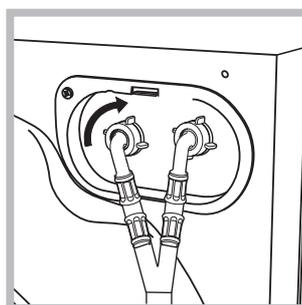
2. Connect the double end hose connection to the washer dryer. Screw connections onto both of the inlet valves located at the top right-hand side at the rear of the appliance making sure the flexible pipe section of the "Y" is not
