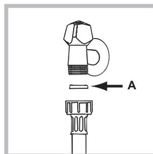
NOTE: the seal is included with the fill hose on UK produced models. So 1 should read.
